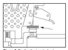
Figure 6. Depth adjustment wheel.
